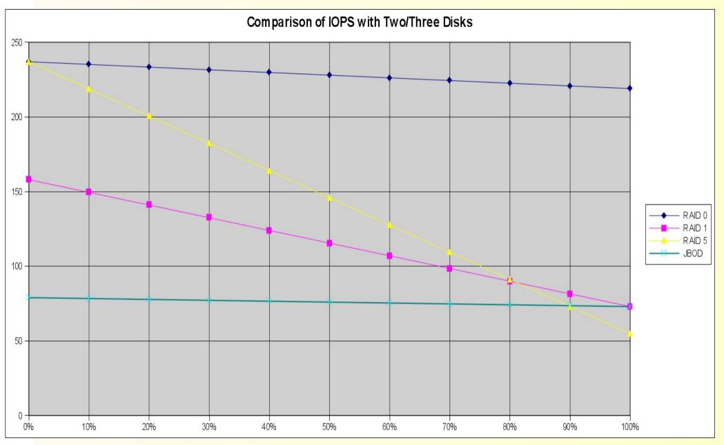
Here we compare a two disk RAID 1 array to a three disk RAID 5 array. RAID 5 manages to maintain a performance advantage.
