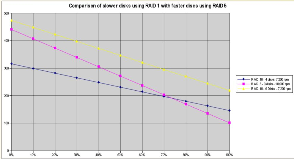
Here we compare a four and six disk RAID 10 arrays using cheaper 7,200 rpm discs with a three disk RAID 5 array of 10,000 rpm.
