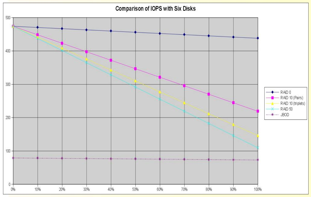
A six disk array of RAID 10 consistently outperforms a six disk array of RAID 50
