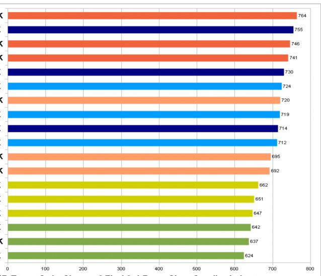
DB Restore based on RAID Type, Strip Size and Firebird Page Size. Smaller is better.
