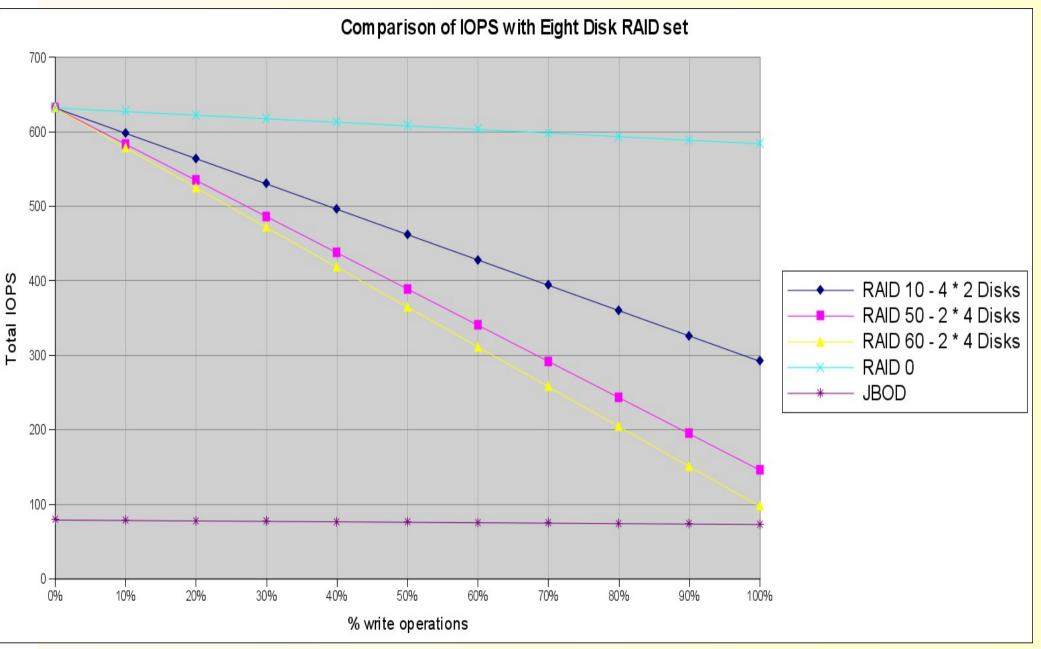
8 disk RAID 10 outperforms all other 8 disk RAID configurations
